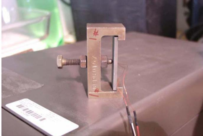
Static stress corrosion specimen with a strain gage on it to measure the applied stress.
