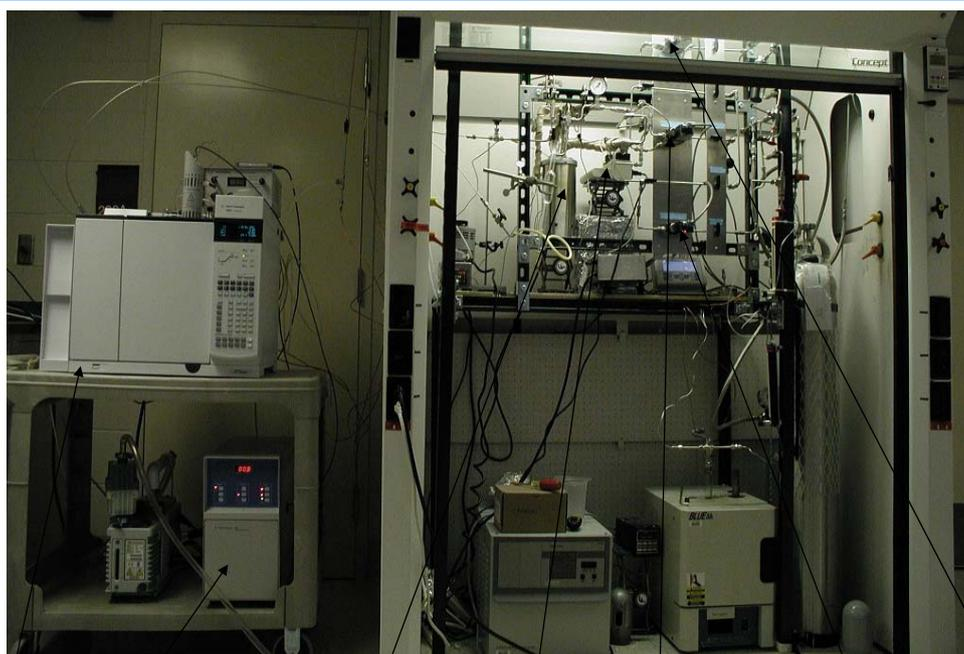
GC SCD Detector    Adsorbent Bed in Furnace    Syringe Pump    N<sub>2</sub>/He MFC    H<sub>2</sub>S in N<sub>2</sub>/He MFC    CO/CO<sub>2</sub> MFC
