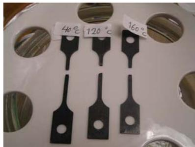
Some of the broken SSRT specimens at different temperatures
