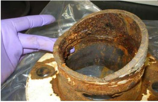
Corroded pipe from an ethanol contact water system
