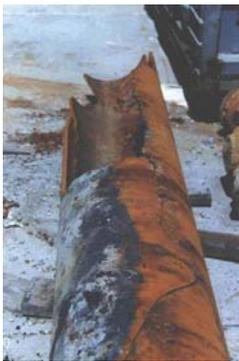
Pitting and Fatigue leading to Pipe Failure - Ductile Iron
