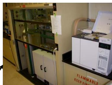
**Gas chromatography (GC) use for online detection of effluent composition**
