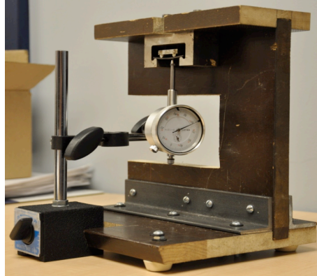
Figure 6. Dial gauge and specimen fixed in the holder for applying definite stress on the sample.
