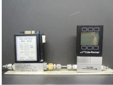
Figure 6. Coupling of flow meters in the experimental setup.
