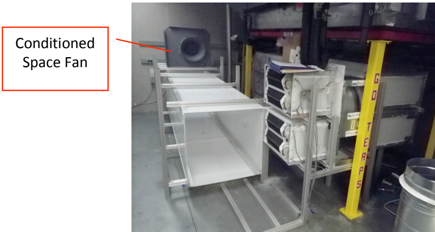
Figure 11. Conditioned space fan.
