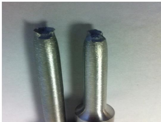
**Figure 7. Broken ductile Al-7075-T6 samples (cup and cone form) after creep experiment at 400°C.**
