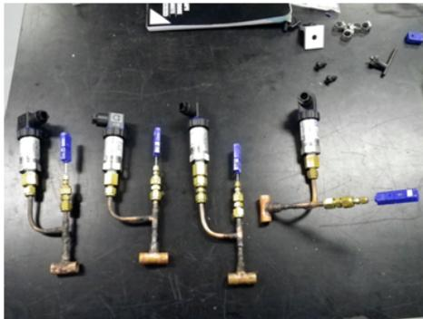
Figure 7. Temperature and pressure modules.
