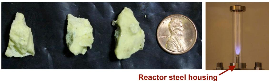
**Figure 19. Large sulfur chunks (left) formed in the burner steel housing (right).**
