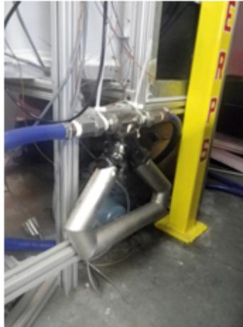
**Figure 4. Water loop mass flow meter.**
